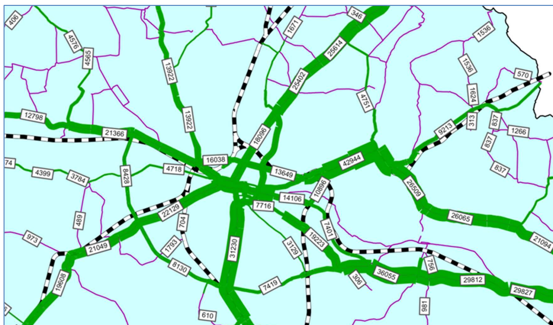
Fig. 2.4. Distribution of traffic volumes of motor vehicles on a typical working day in 2015 in the city of Bydgoszcz [Study, 2016]
